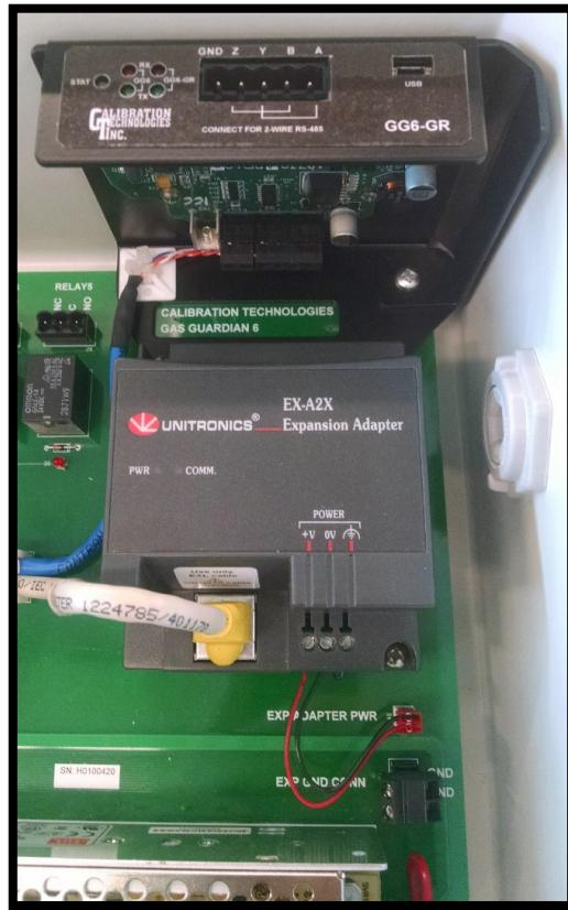
4. Cut the zip ties along the Expansion Adapter communication cable, and install the new communication/power cable alongside the Expansion Adapter cable.
