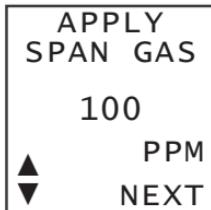
Apply Certified Calibration Gas at 0.3 to 1.0 L/minute. Once the output signal has peaked (or 2 minutes maximum), press the  $\Delta$  /  $\nabla$  keys to change the value on display to match the value of the Certified Calibration Gas.
